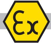
Marking to ATEX 94/9/EC Directive:  $\text{Ex}$  II 2 G Ex d IIC T6 or T5 Gb / II 2 D Ex tb IIIC T80°C or T95°C Db IP6X
