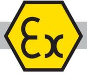
Marking to ATEX 94/9/EC Directive:  $\text{Ex}$  II 2 G Ex d IIC T4 or T3 Gb / II 2 D Ex tb IIIC T126°C or T141°C Db IP66
