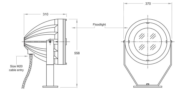
Dimensions shown are within manufacturing tolerances. Floodlight weight: 22 KG. All dimensions are in mm.
