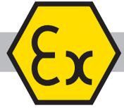
Marking to ATEX 94/9/EC Directive:  $\text{Ex}$  II 2 G Ex d IIB T6 Gb / II 2 D Ex t IIIC T80°C Db IP6X
